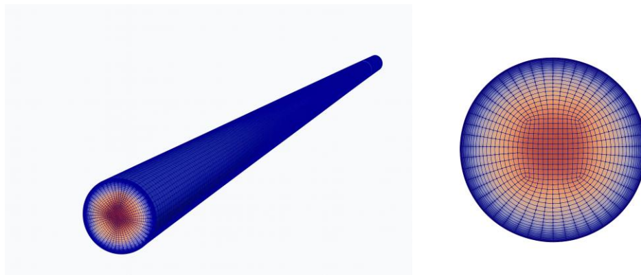
Fig 2: Mesh generation view using blockMesh
